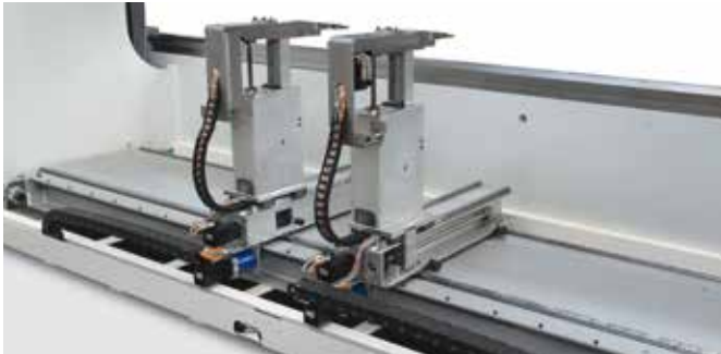
Top view standard three-point gauging finger
