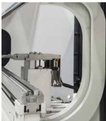
Increase the table-ram/stroke/gap distance in 100 mm steps
